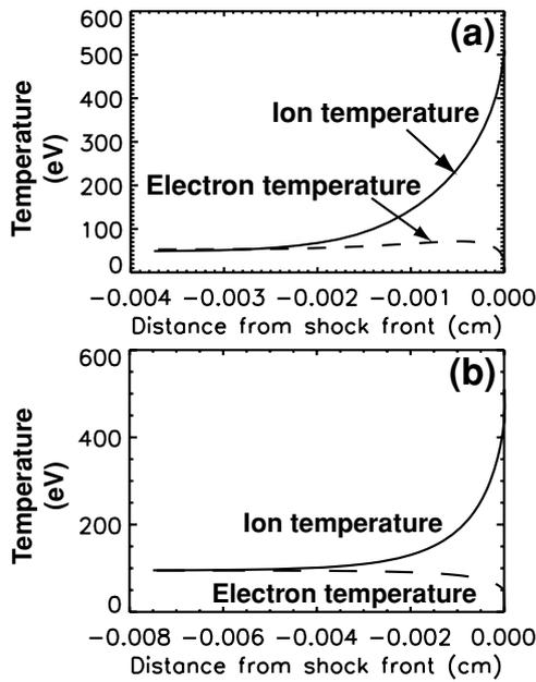
**Fig. 3** Ion and electron temperatures behind the shock front for the parameters from the experimental system, assuming a shock moving at 150 km/sec. The shock front is located at 0 cm. (a) Temperature profiles with only collisional heat exchange. (b) Temperature profiles with both collisional heat exchange and radiative cooling of the electrons. In this system, radiative cooling becomes important before collisional heat exchange can equilibrate the electron and ion temperatures
