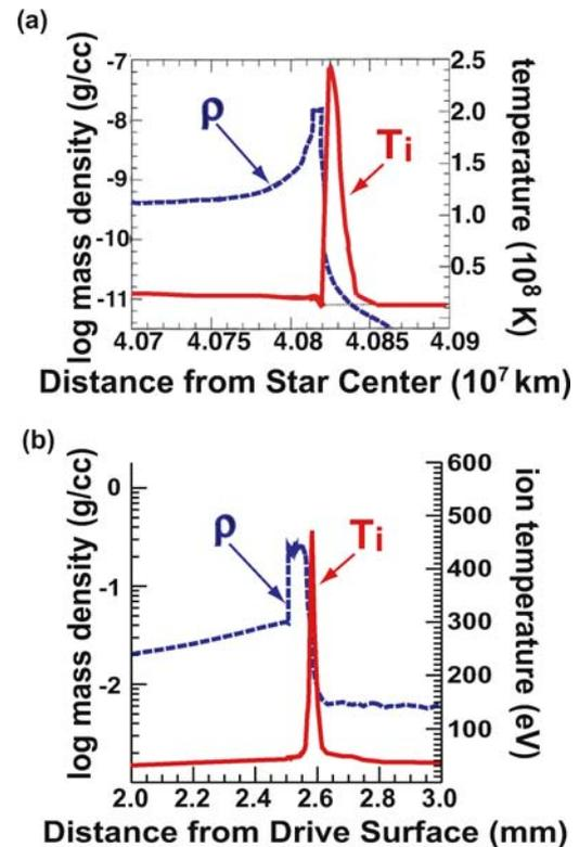
**Fig. 2** 1D Lagrangian simulations of the two systems discussed. (a) 1D VISPHOT calculation adapted from Ensmann and Burrows (1992). (b) 1D Hyades simulation of discussed experimental system. Both systems show a layer of highly compressed material accompanied by quick cooling through a region that is thin compared to the distance the shock has traveled
