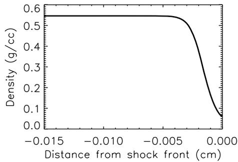
**Fig. 4** Density profile when affected by radiation losses. In this simple analytic model, the radiative transfer equation was not fully employed, nor was the influence of increasing opacity as electron temperature decreased. Both these factors would affect the final density of the cooling layer. Here, the final density is dictated by the loss of all electron energy via radiation
