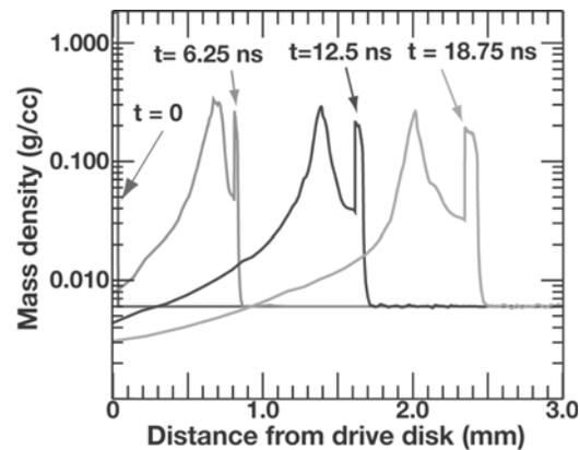
**Figure 3.** The density profile at several times, from a simulation using HYADES for a  $40 \mu\text{m}$  Be drive disk. The thin dense layer to the right is the shocked Xe, while the peaked structure to the left is the drifting Be.
