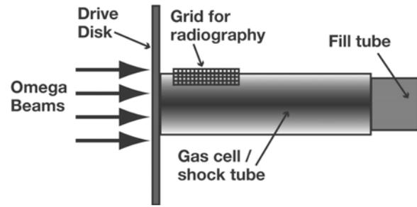
**Figure 2.** Sketch of experiment to produce radiative shocks. The tube is filled with Xe at  $6 \text{ mg/cm}^3$ . The xray source for radiography is below the page, and the detector is above the page.
