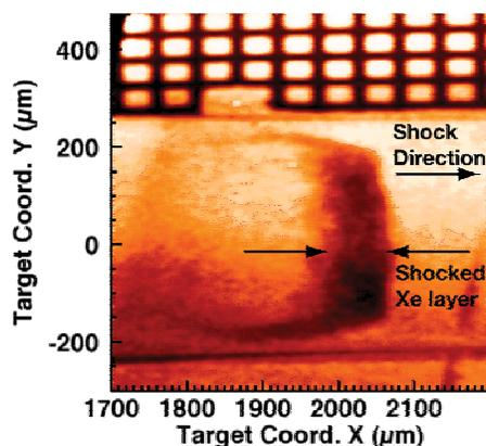
**Figure 4.** Radiographic data, at 14.6 ns after the initiation of an experiment using a 20  $\mu\text{m}$  Be drive disk. The image is stretched for clarity, the grid cells are squares spaced 63  $\mu\text{m}$  from center to center.
